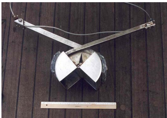
Fig. 10. Van Veen grabber to take samples from sea bottom / soil. Sample size ~1 kg.
