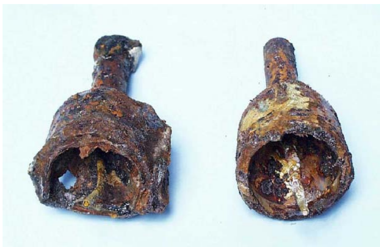
Fig. 3. Recovered anti-tank rounds. The corrosion already removed parts of the metal casing.
